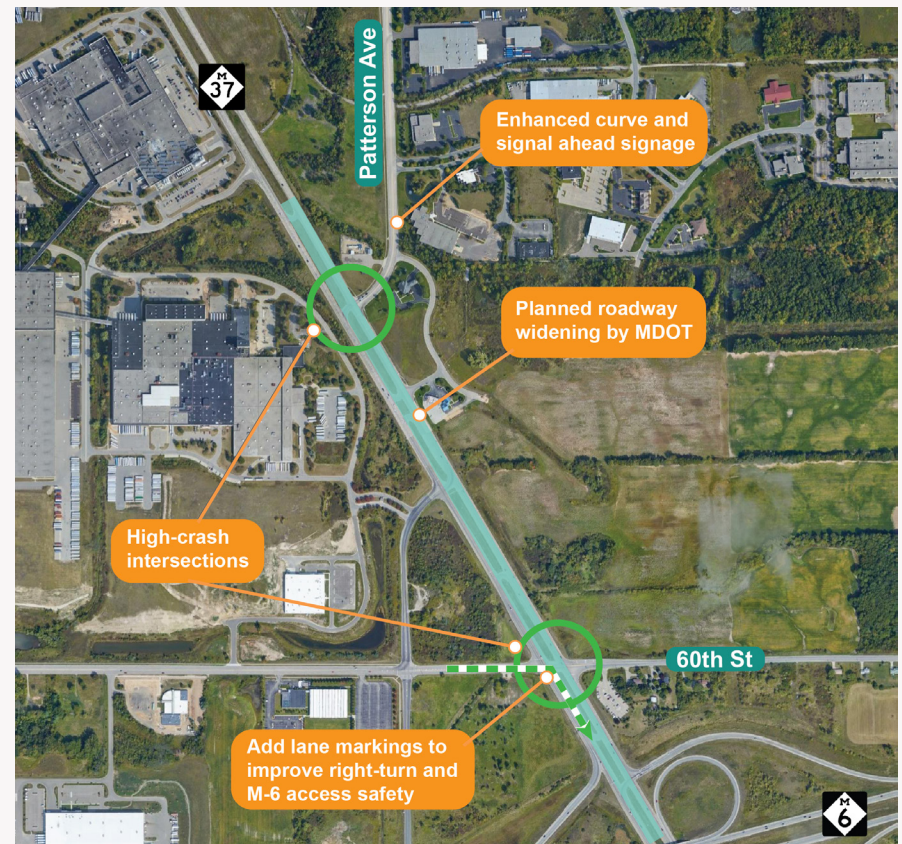
Proposed M-37/Patterson Avenue/60th Street Safety Enhancements
