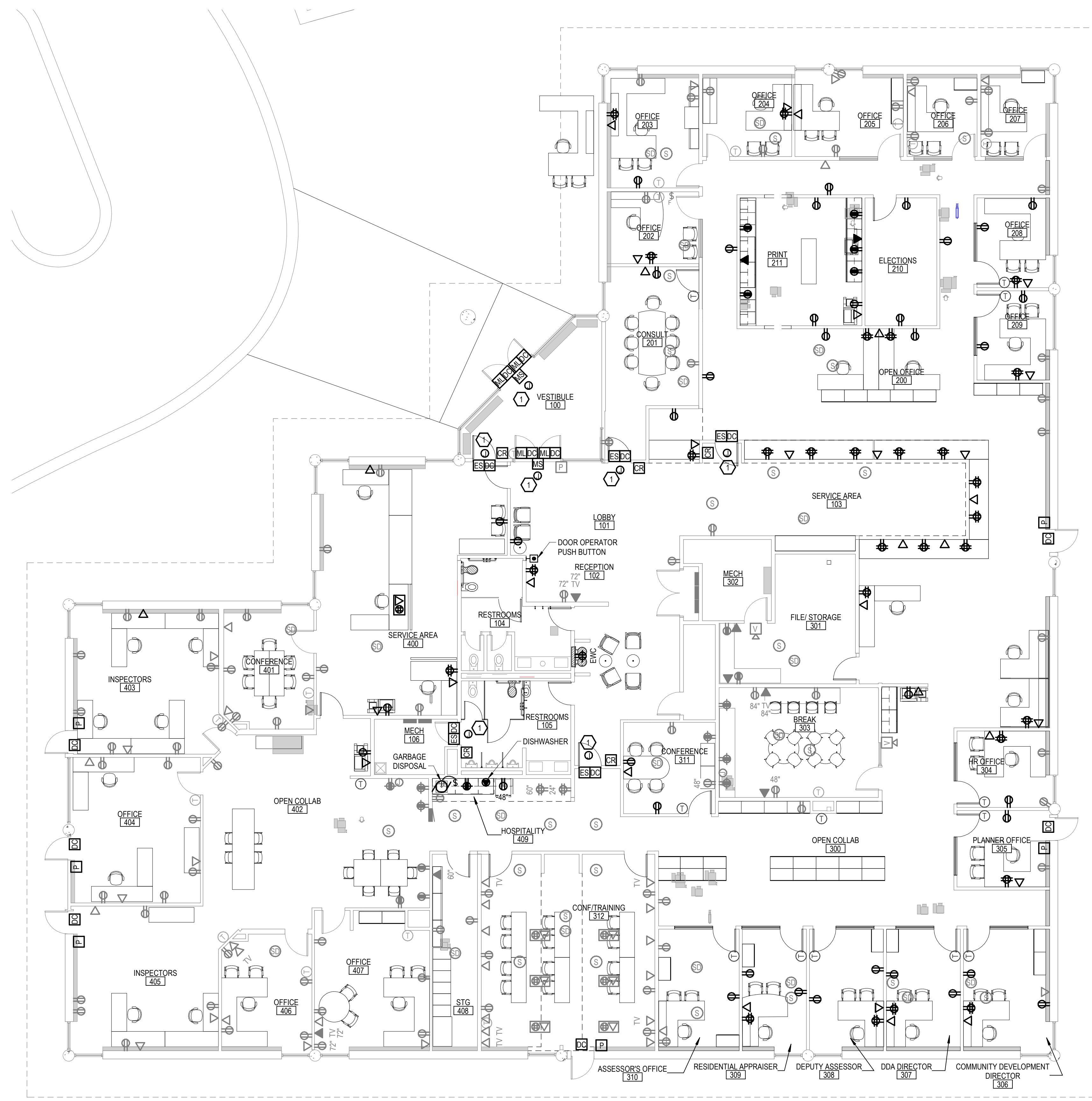
FIRST FLOOR POWER AND SYSTEMS PLAN 1/8" = 1'-0"
