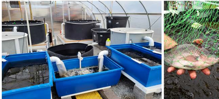
Fish waste in the tanks (rear) flows into clarifiers (center) to separate the solids from the nitrites. Microbes on floating biofilters (foreground) consume the nitrites and convert them to nitrates for the plants to absorb. Greenhouse-raised tilapia on right (inset).
