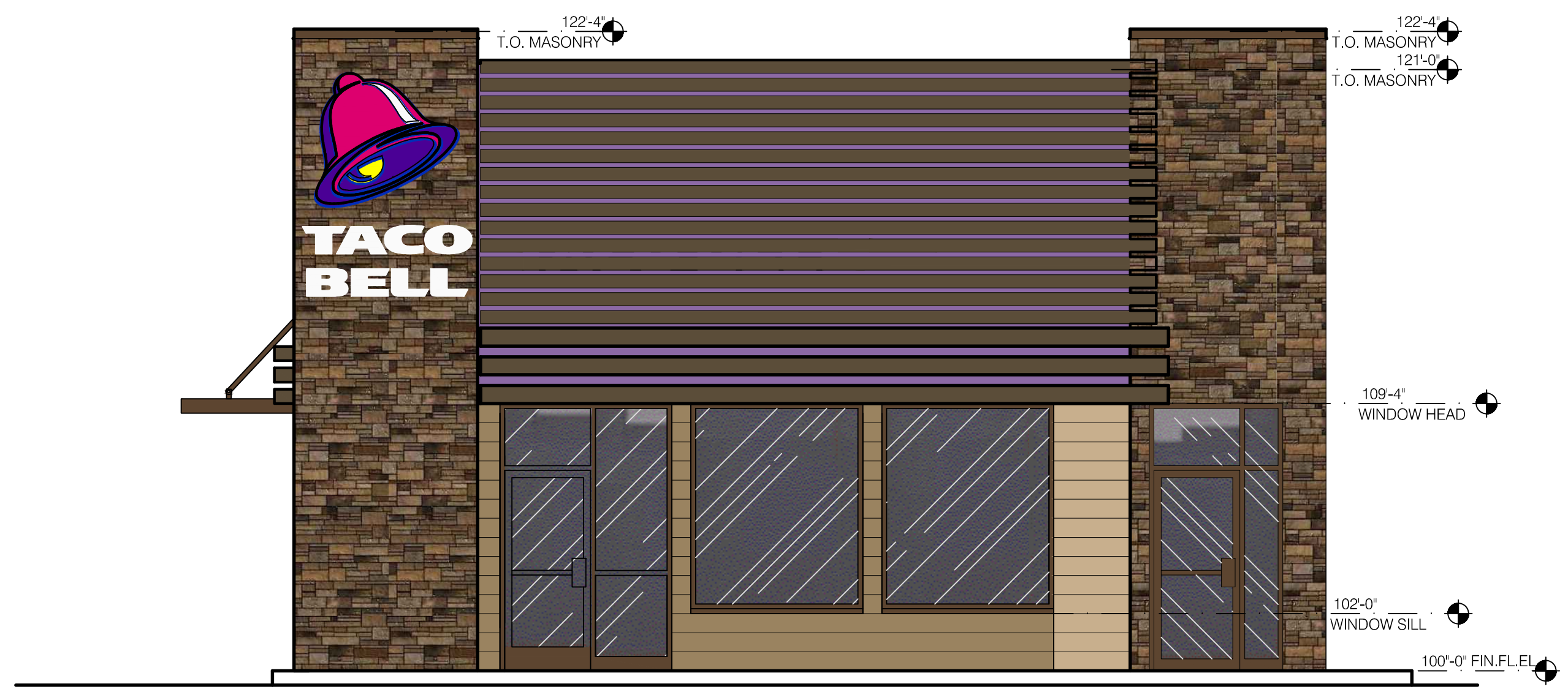
3 NORTH EXTERIOR ELEVATION A4.0 SCALE: 1/4" = 1'-0"
