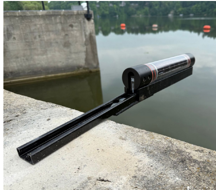
▲ The reader sits on top of the dam and reads the water level for the impoundment area (behind the dam).
